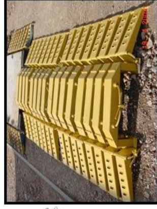
Ramp section engaged on to the rail.
